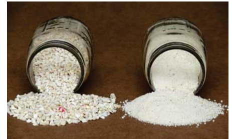
Regrind at a PVC pipe plant for inclusion into making new pipe.
