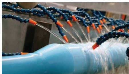
In-line process for manufacturing PVCO pipe.
