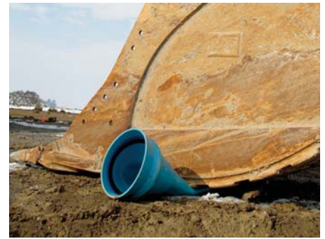
Toughness of PVCO pipe to withstand crushing.
